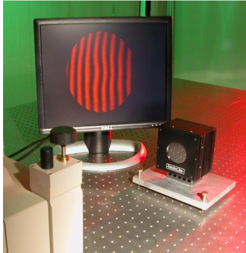
Figure 12. Example of a 349-channel Photonex deformable mirror. The aperture of only 53 mm is substantially smaller than a conventional deformable mirror which has a 160 mm aperture
