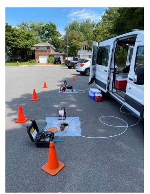
Typical set-up of Northrop Grumman/US Navy groundwater sampling operations on a residential street.
